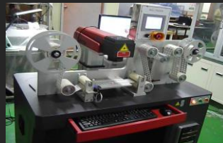
Product Name : Label Marking (Roll To Roll 시스템)
